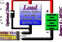
**Operation:** The small red **LED** on the **NERS** lights up when the **NERS** turns the output ON. If the **NERS** stops receiving a good signal from the receiver (occurs if there is any radio interference or if you turn off your transmitter) it will hold the last state (ON/OFF) indefinitely until it sees a valid signal again. If your radio system has a failsafe setting, then you can use that to set what the **NERS** will do in case of a lost signal.
